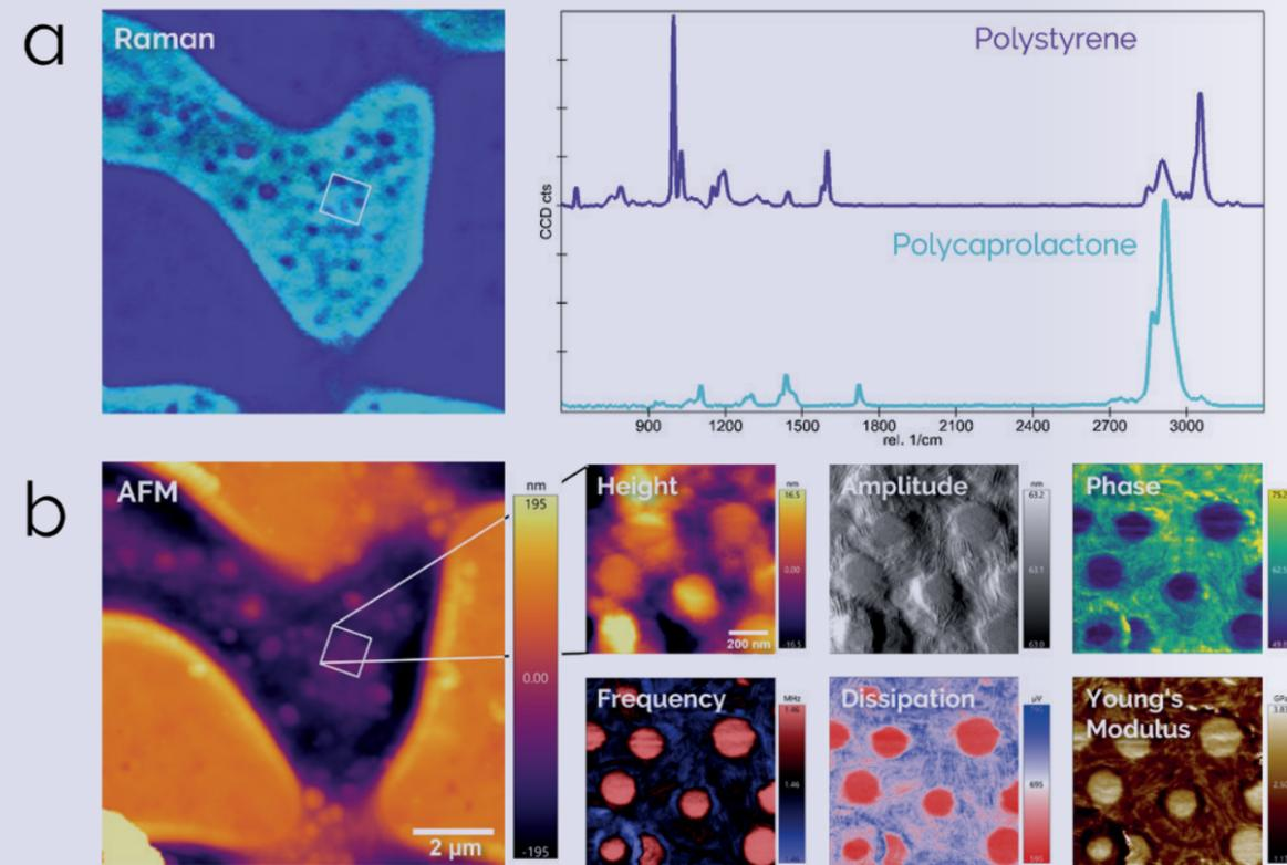
**Figure 3:** (a) Raman imaging of a polymer blend of polystyrene (PS) and polycaprolactone (PCL). The two phases of PS (purple) and PCL (cyan) are clearly distinguishable by their Raman signals, and are colour coded according to their corresponding spectra. (b) AFM topography (AC mode) of the same region measured in (a). The zoomed-in panels reveal additional information on the more heterogeneous parts of the polymer mixture, including an estimation of Young's modulus (AM-FM).
