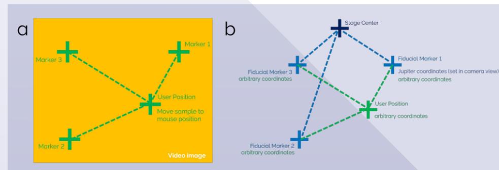
**Figure 1:** (a) TrueOrigin's video image-based coordinate system. (b) Ergo Advanced Automation's coordinate system, based on a transformation between two sets of three coordinates.
